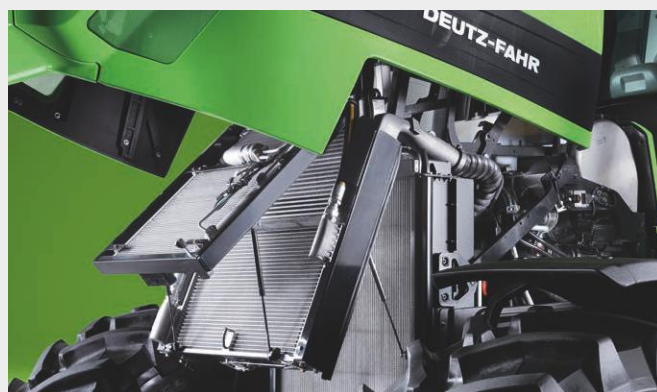
↑ The engine radiator can be opened and cleaned easily.
